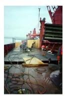
Third, the ship was ballasted to prevent it from moving on the seabed and to start the preliminary unloading of hold No. 4, which contained a mixture of water and clinker. At the same time, plates were welded to the ship at different locations to reinforce it and prevent it from splitting in two.
